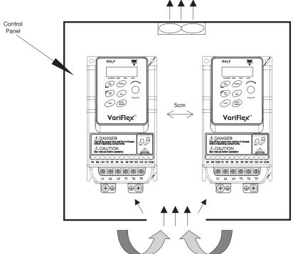
The necessary physical space and cooling should be provided, based on the ambient temperature and the heat loss in the panel.
